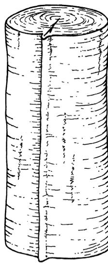
a. Blunt-nosed rib showing occluded crack covered by intact annual rings
