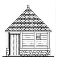
The designs have been drawn up and the various planning consents and Faculties obtained. A composting toilet functions without heat or water. It is cheap to run and maintain and is environmentally sustainable. The substantial, detached building design is based on traditional lines employing local materials and erected on the site of a former stone toilet.
